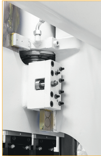
3 point guiding system with ball bearings
