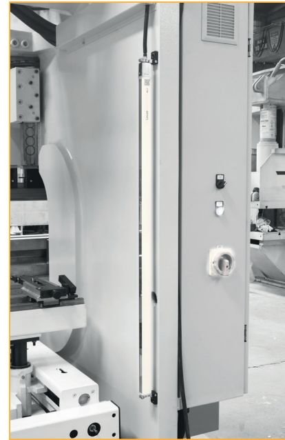
Back light curtain safety system
